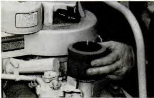
ENGINE FLOODING can often be traced to a dirty air cleaner. Dirty filters will shorten engine life
